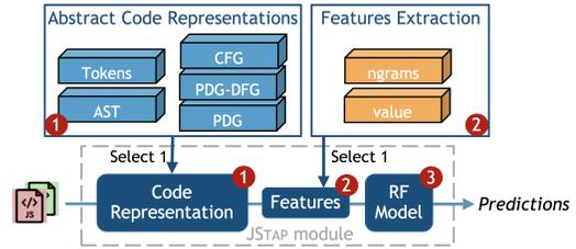
Figure 1: Architecture of JSTAP with focus on one module
